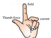
➡ The magnetic force exerted on a current-carrying wire placed in a uniform magnetic field.
